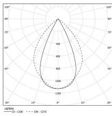
Beam angle Wide flood 80° Application Weight
