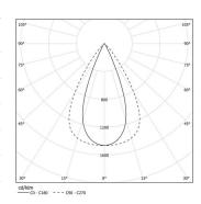
Beam angle Flood 65° Application Weight
