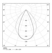
Beam angle Wide flood 80° Application Weight
