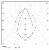
Beam angle Wide flood 80° Application Weight
