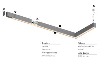
3000K Light Source Luminaire 27W 32,9W Power 4900lm 2300lm Flux Efficiency 1811m/W 70lm/W LOR 47% -UGR <25 -
