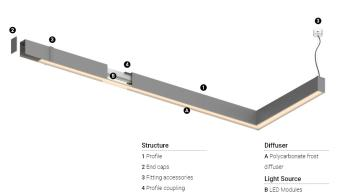
4000K Light Source Luminaire 24W 29,3W Power 2130lm 4530lm Flux Efficiency 189lm/W 73lm/W LOR 47% -UGR <25 -
