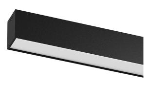
Design: Eduardo Souto de Moura Surface or pendant luminaire with housing made of aluminium profile with 25micron maximum corrosion resistance anodization with matt finish or with textured electrostatic 100% polyester paint. Frosted polycarbonate diffuser with user friendly clipping system and double fitting system: flushed or
