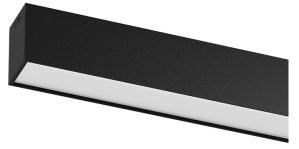
Design: Eduardo Souto de Moura Surface luminaire with housing made of aluminium profile with 25micron maximum corrosion resistance anodization with matt finish or with textured electrostatic 100% polyester paint. Frosted polycarbonate diffuser with user friendly clipping system. Aluminium anodised end caps with matt finish or
