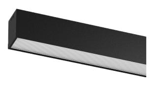
Design: Eduardo Souto de Moura Surface or pendant luminaire with housing made of aluminium profile with 25micron maximum corrosion resistance anodization with matt finish or with textured electrostatic 100% polyester paint. Prismatic polycarbonate diffuser with low luminance and glare control (UGR<19 for low output or UGR<22 for High Output).
