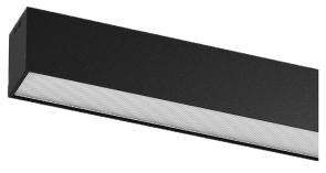
Design: Eduardo Souto de Moura Surface or pendant luminaire with housing made of aluminium profile with 25micron maximum corrosion resistance anodization with matt finish or with textured electrostatic 100% polyester paint. Prismatic polycarbonate diffuser with low luminance and glare control (UGR<19 for low output or UGR<22 for High Output).
