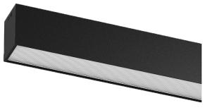
Design: Eduardo Souto de Moura Surface or pendant luminaire with housing made of aluminium profile with 25micron maximum corrosion resistance anodization with matt finish or with textured electrostatic 100% polyester paint. Prismatic polycarbonate diffuser with low luminance and glare control (UGR<19 for low output or
