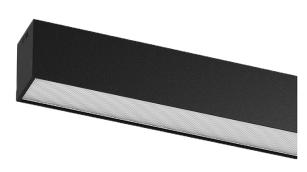
Design: Eduardo Souto de Moura Surface or pendant luminaire with housing made of aluminium profile with 25micron maximum corrosion resistance anodization with matt finish or with textured electrostatic 100% polyester paint. Prismatic polycarbonate diffuser with low luminance and glare control (UGR<19 for low output or UGR<22 for High Output).
