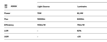
Beam angle Diffuse Application Application Weight 5,2Kg
