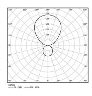
Beam angle Diffuse Direct/ Indirect
