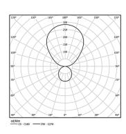
Beam angle Diffuse Direct/ Indirect
