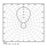
Beam angle Diffuse Direct/ Indirect
