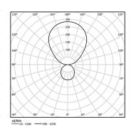
Beam angle Diffuse Direct/ Indirect
