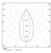
Beam angle Elliptical 22×47° Application Weight
