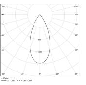
Beam angle Flood 46° Application Weight
