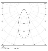
Beam angle Flood 46° Application Weight
