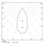
Beam angle Flood 46° Application Weight
