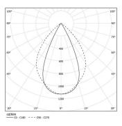
Beam angle Wide flood 80° Application Weight
