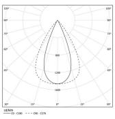
Beam angle Flood 65° Application Weight
