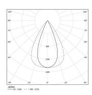
Beam angle Flood 65° Application Weight
