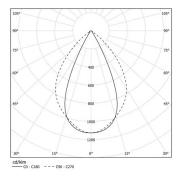
Beam angle Wide flood 80° Application Weight
