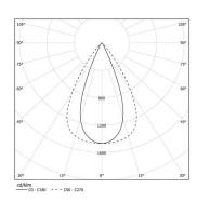
Beam angle Flood 65° Application Weight
