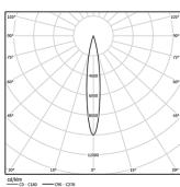
Beam angle Spot 15° Application Weight 0,64Kg
