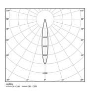
Beam angle Spot 15° Application Weight 0,64Kg
