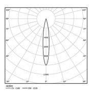
Beam angle Spot 15° Application Weight 0,64Kg
