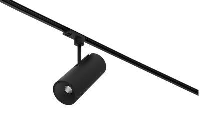
Design: O/M + Bartenbach GmbH Track-mounted spotlight with die-cast aluminium body with electrostatic 100% polyester paint finish. Spot-lens with individual complex surface rips to provide a focal light and an extremely narrow beam. Orientable by 90° horizontal rotation and 330° vertical rotation. Driver included.
