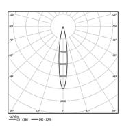
Beam angle Spot 15° Application Weight 0,64Kg
