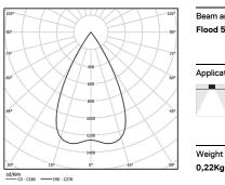
Beam angle Flood 56° Application Weight
