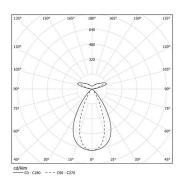
Beam angle Flood 64° / batwing
