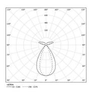
Beam angle Flood 64° / batwing
