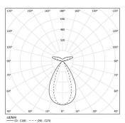
Beam angle Flood 64° / batwing
