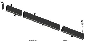
1 Profile 2 End caps 3 Fitting accessories 4 Profile coupling Modules A inFinit module (middle) B inFinit module (end) C Indirect module
