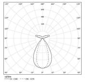
Beam angle Flood 64° / batwing Application
