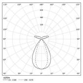
Beam angle Flood 64° / batwing Application
