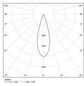
Beam angle Medium 31° Application Weight 1,8Kg
