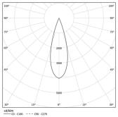
Beam angle Medium 31° Application Weight 1,8Kg
