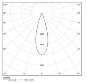
Beam angle Medium 31° Application Weight 1,8Kg
