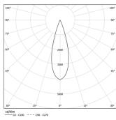
Beam angle Medium 31° Application Weight 1,8Kg
