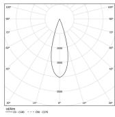
Beam angle Medium 31° Application Weight 1,8Kg
