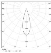
Beam angle Medium 31° Application Weight 1,9Kg
