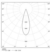
Beam angle Medium 31° Application Weight 1,3Kg
