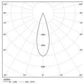
Beam angle Medium 31° Application Weight 2,5Kg
