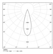
Beam angle Medium 30° Application Weight 0,6Kg
