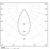
Beam angle Flood 50° Application Weight 0,6Kg
