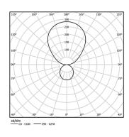
Beam angle Diffuse Direct/ Indirect
