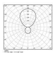
Beam angle Diffuse Direct/ Indirect
