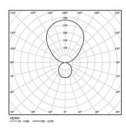
Beam angle Diffuse Direct/ Indirect
